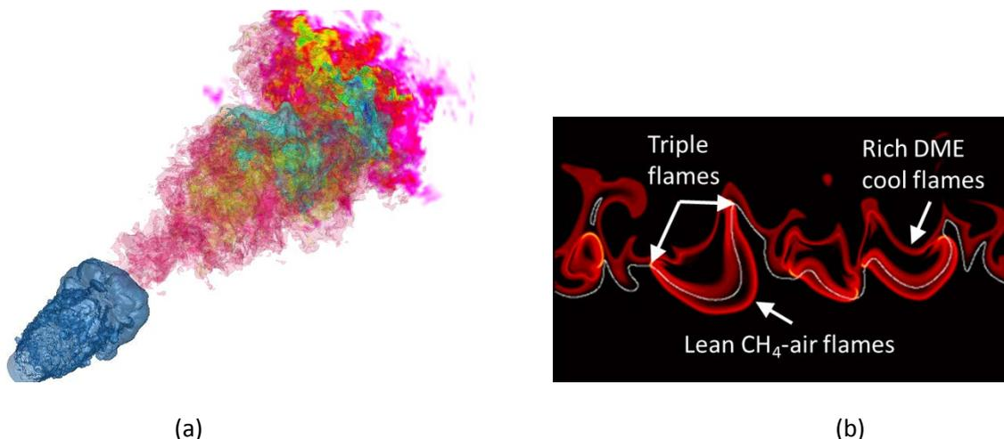
Figure 1: (a) Volume rendering of jet fluid mass fraction from two consecutive injection pulses (first pulse shaded red-green, second pulse shaded blue). (b) Instantaneous heat release colour map from Direct Numerical Simulation of lean methane-air flame ignited by injection of the bio-derived diesel-substitute, dimethyl-ether.
