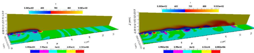
Figure 1: Characteristics of the transition from subcritical to supercritical regime in high speed spray flows at different time instants (a)  $t = 0:004ms$  (b)  $t = 0:02ms$ .
