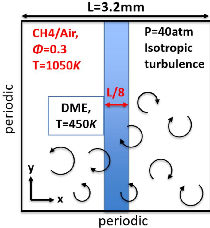
The computational domain with DME and methane-air mixture
