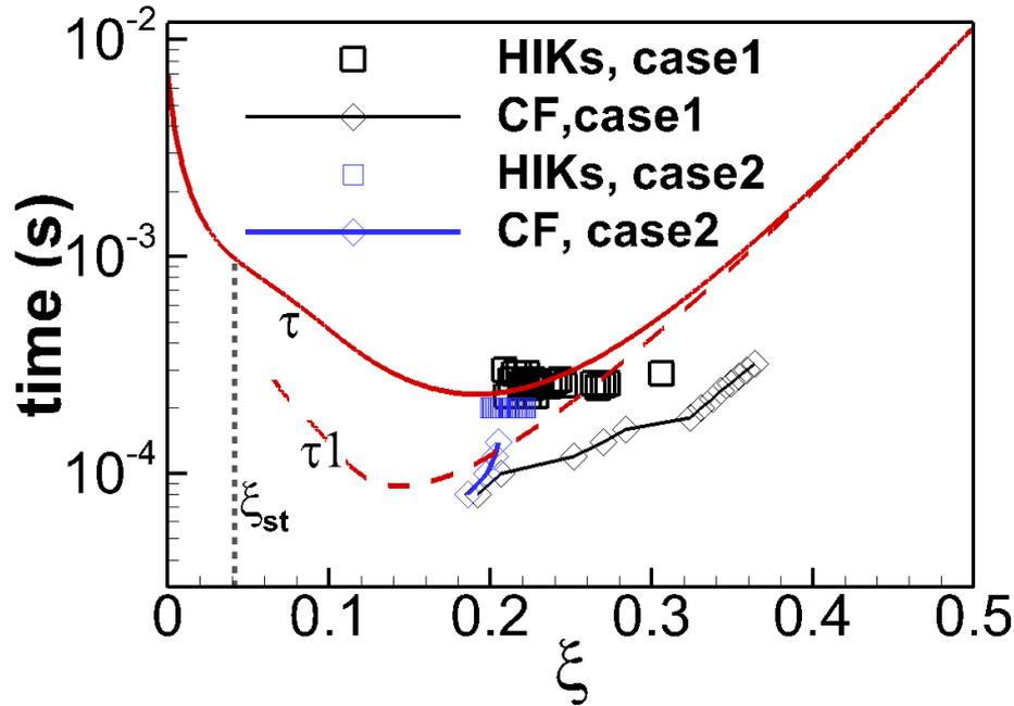
Time of HIKs compared with homogeneous ignition delay times
