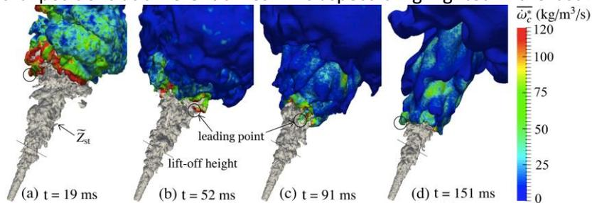
the 3D trajectory of the leading point from its initial location to the final lift-off height for two flames, F1 and F2, with different jet exit velocities. The leading point trajectory seems to follow a spiral-shape for both F1 and F2 flames.
