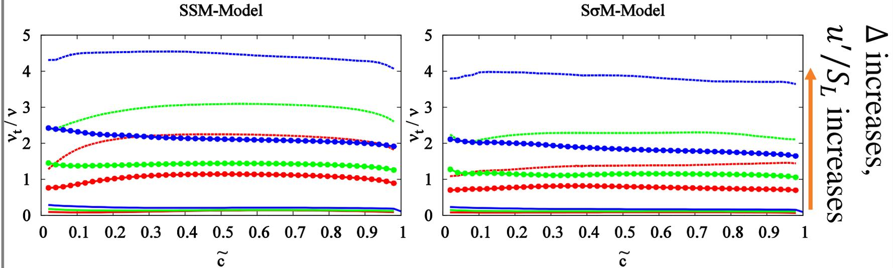
Comparison of the mean values of normalised turbulent viscosities obtained from the SSM and the sigma Model SσM conditional on  $\tilde{c}$ .
