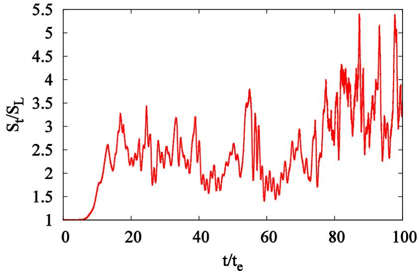
Variation of turbulent flame speed over time for an IO configuration. Inflow velocity is a filtered version of  $S_T$ .
