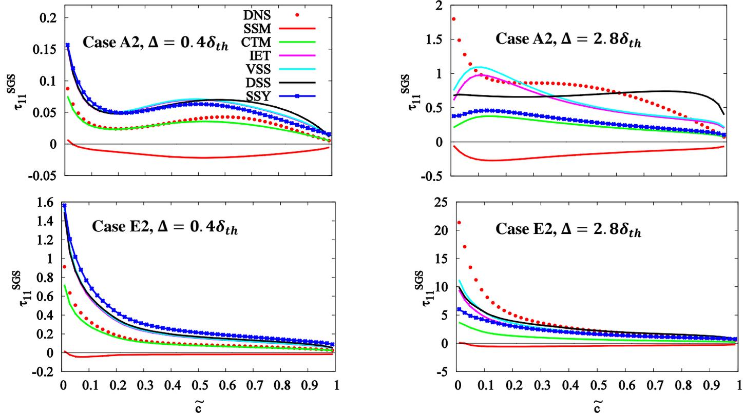
Conditional plot of  $\tau_{11}^{SGS}$  from DNS as well as different model expressions against  $\tilde{c}$  for filter width  $\Delta \approx 0.4\delta_{th}$ ,  $\Delta \approx 2.8\delta_{th}$  for cases A2 (left) and E2 (right).
