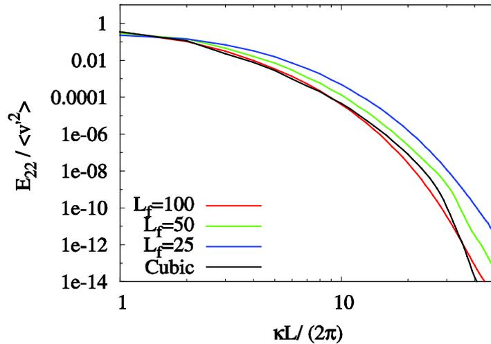
One dimensional energy spectra using the filtered forcing method in comparison to the unfiltered forcing in a cubic domain.
