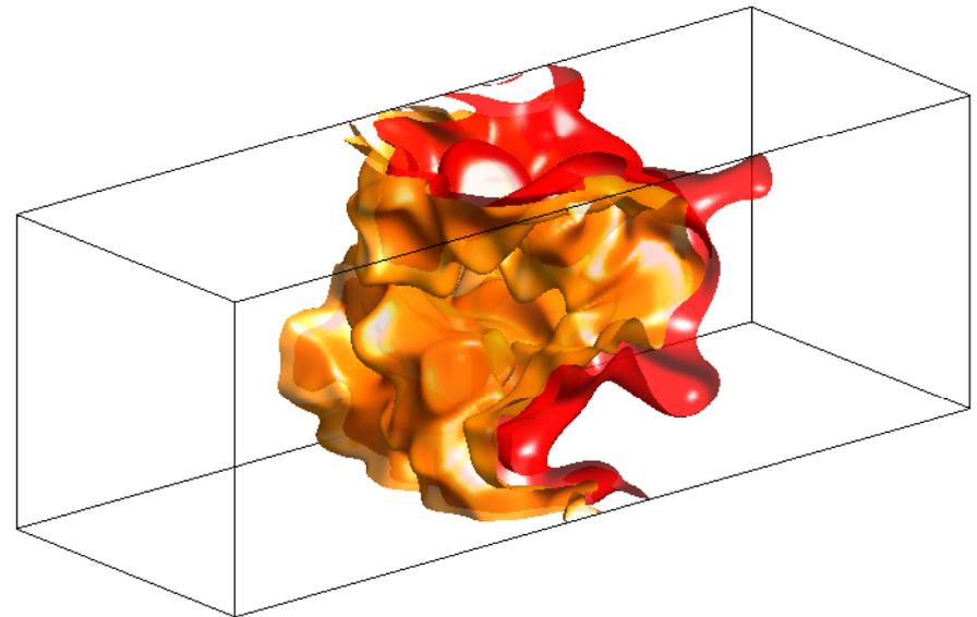
Planar flame with filtered forcing applied to the unburned gas side only.
