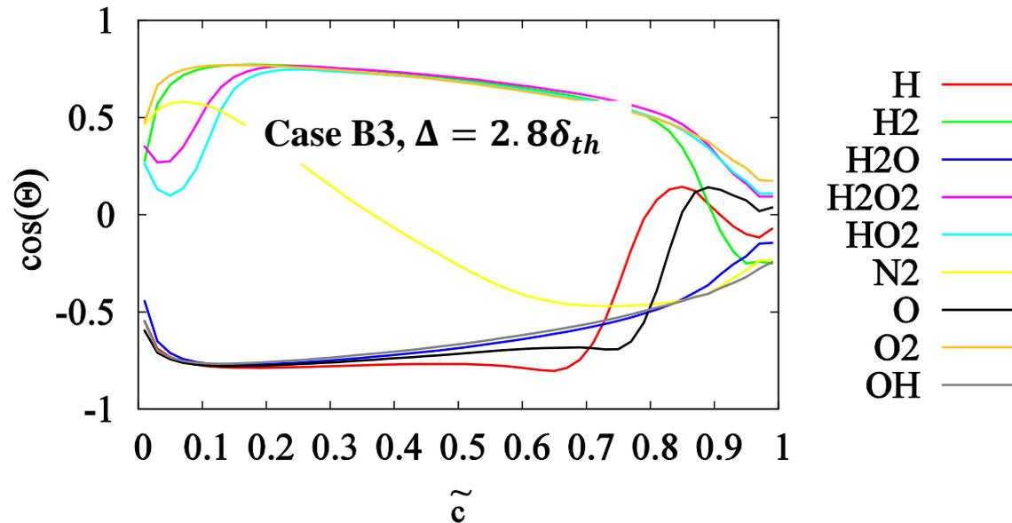
Cosine of the angle  $\Theta$  between  $\bar{\rho}(u_i \widetilde{Y}_m - \tilde{u}_i \widetilde{Y}_m)$  for different species  $m$  calculated from DNS and  $-\partial \widetilde{c}_T / \partial x_i$  predictions conditional on  $\tilde{c}$  for case B and filter width  $\Delta \approx 2.8\delta_{th}$ .
