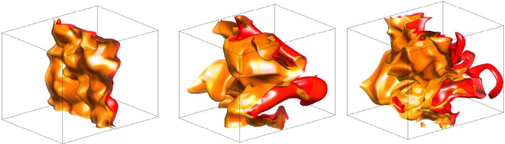
Instantaneous view of  $c$  isosurfaces for cases A2, D2 and E2 at  $t = \delta_{th}/S_L$ . The value of  $c$  increases from 0.1 to 0.9 from yellow to red.
