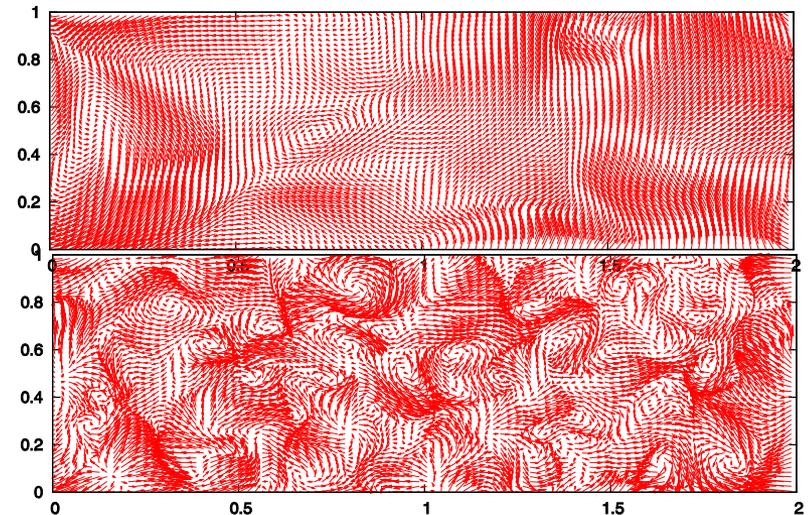
Instantaneous velocity field in a rectangular domain with a high pass filtered forcing term of characteristic length  $L_f = L$  (top)  $L_f = L/4$  (bottom).
