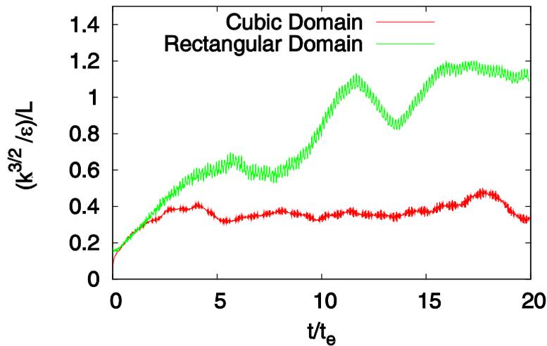
Development of the normalized length scale  $(k^{3/2}/\epsilon)/L$  with non-dimensional time  $t/t_e$  in a cubic domain and a rectangular domain, for an isothermal Lundgren-forced flow.
