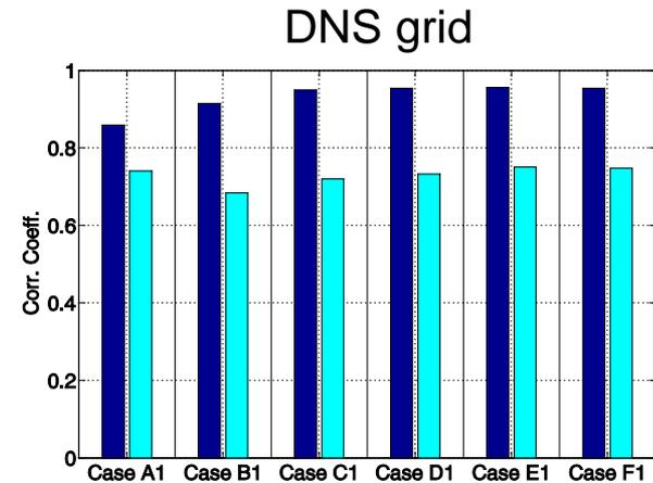
Correlation coefficients between modelled and the corresponding value extracted from DNS: CTM (■); YOS (■); DSS (■);
