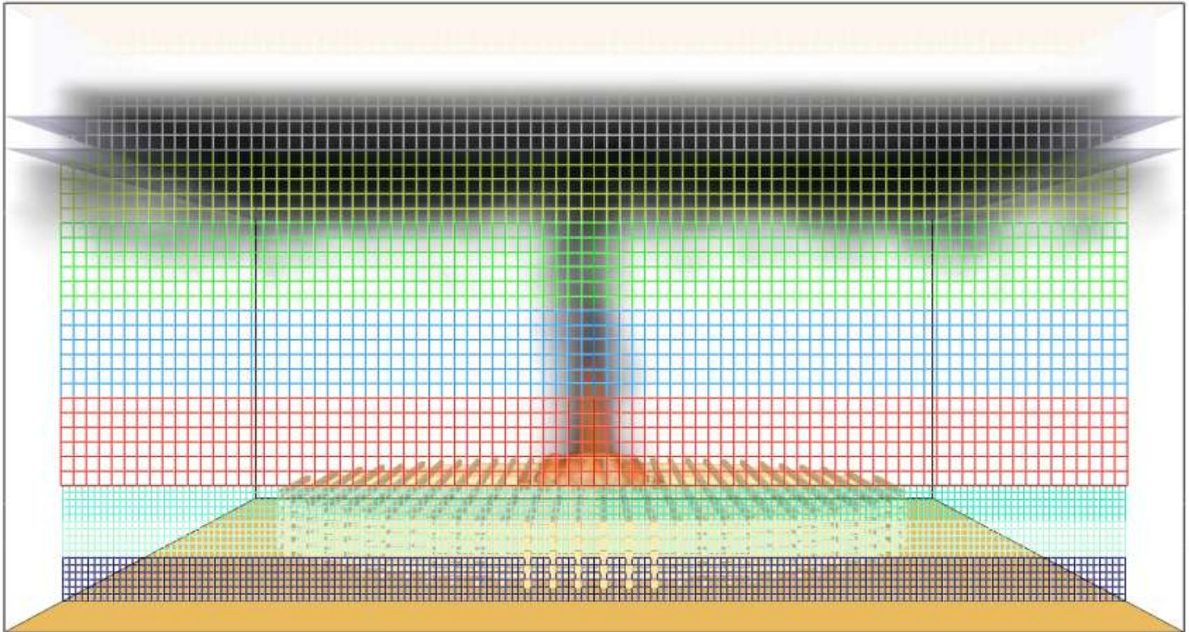
MPI used, 11 meshes in total, cell size **0.03m×0.03m×0.035m** (to fit per cell - per cross section) for wood sticks; cell size **0.06m×0.06m×0.07m** for upper flame and ceiling part; total number of cells 670 320
