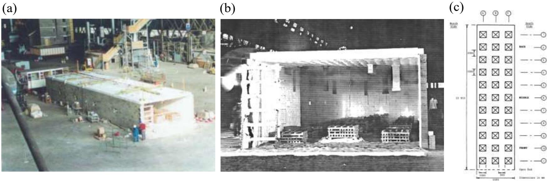
**Fig. 1. (a): Test compartment of the BST/FRS 1993 Fire Test Series (22.8m × 5.6m × 2.75m); (b): Ignition of the first row of wood cribs in test number 2, front view; (c): Layout of the wood cribs distribution within the test compartment in plan view.**
