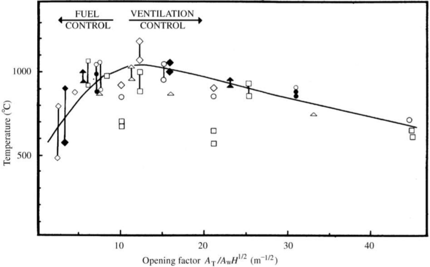
**Figure 10.6** Average compartment temperatures during the steady burning period for wood crib fires in model enclosures as a function of the ‘opening factor’  $A_T/A_w H^{1/2}$ . Symbols refer to different compartment shapes (see Table 9.3): ○, 1 × 2 × 1; △, 2 × 2 × 1; ◇, 2 × 1 × 1; □, 4 × 4 × 1. Solid points are means of 8–12 experiments (Thomas and Heselden, 1972). Reproduced by permission of The Controller, HMSO. © Crown copyright
