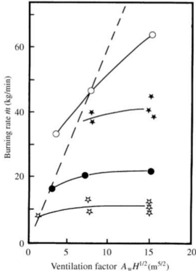
**Figure 10.2** Variation of mass burning rate with  $A_w H^{1/2}$  for large ventilation openings and different fire loads (wood cribs):  $\star$ , 7.5 kg/m<sup>2</sup>;  $\bullet$ , 16 kg/m<sup>2</sup>;  $\blackstar$ , 30 kg/m<sup>2</sup>;  $\circ$ , 60 kg/m<sup>2</sup>. Dashed line (— —) represents Equation (10.1) for the ventilation-controlled fire (Thomas *et al.*, 1967a). Reproduced by permission of The Controller. HMSO. © Crown copyright
