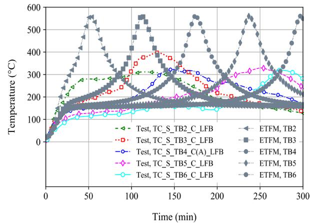
(b) TB2, bottom flange beam temperature
