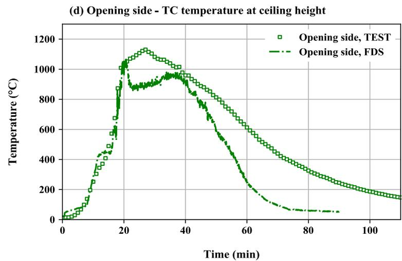
Comparison of thermocouple (TC) temperatures between test and model
