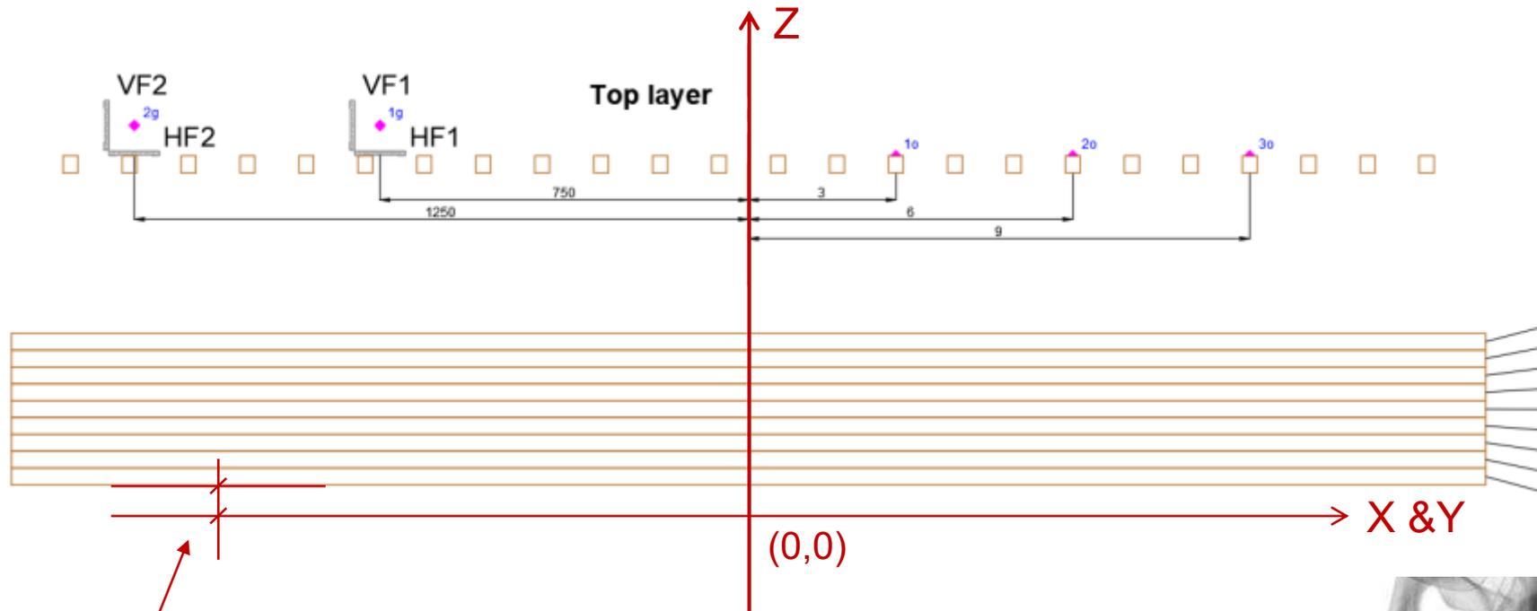
50mm offset for the ignition burner & steel tubes
