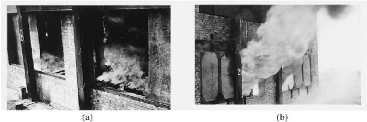
**Figure 10.7** The effect of a large exposed fuel surface area on fire behaviour. (a) Fuel control regime,  $15 \text{ kg/m}^2$ . Fuel in the form of wood cribs,  $A_f = 55 \text{ m}^2$ : no external flaming. (b) Ventilation control regime,  $7.5 \text{ kg/m}^2$ . Fuel was fibre insulating board, lining the walls and ceiling,  $A_f = 65 \text{ m}^2$ ; external flaming lasted for 5.5 minutes (Butcher *et al.*, 1968). Reproduced by permission of The Controller, HMSO. © Crown copyright
