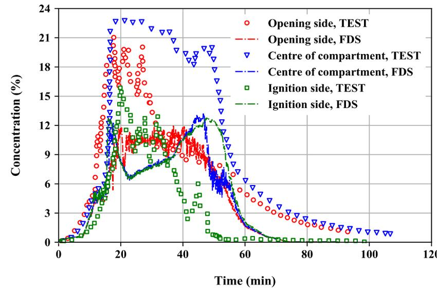
**Comparison of gas concentrations between test and model (oxygen concentration test data at rear compartment invalid after 7 mins, due to pipe leakage)**
