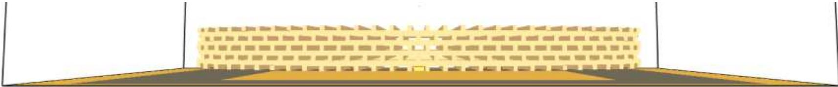
Now every 2 layers we have the **wood sticks ‘offset’ in parallel distance of 60mm**, to generate higher porosity for FDS model, v4 series. Multi-mesh shown below.
