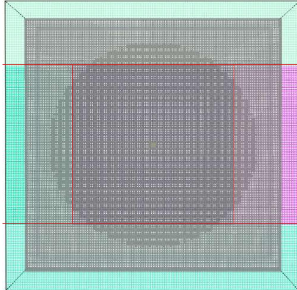
Multi-mesh in elevation view, mesh number 30 in total, cell size **0.03m×0.03m×0.035m** (to fit per cell - per cross section) for wood sticks, total number of cells 2,201,472 (HPC on ARCHER via UKCTRF)
