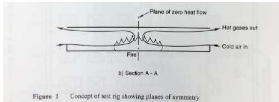
Figure 1 Concept of test rig showing planes of symmetry
