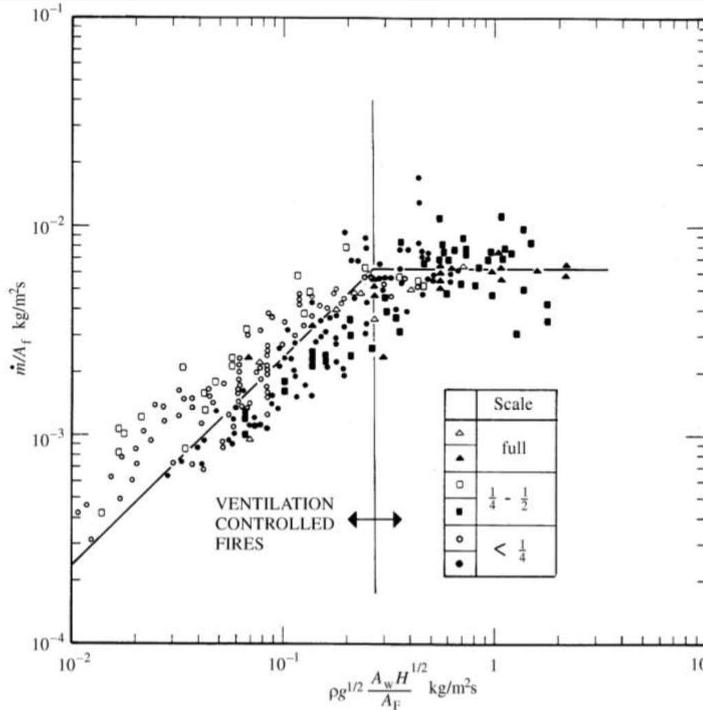
**Figure 10.5** Identification of the transition between ventilation-controlled and fuel-controlled burning for wood cribs, according to Harmathy (1972)
