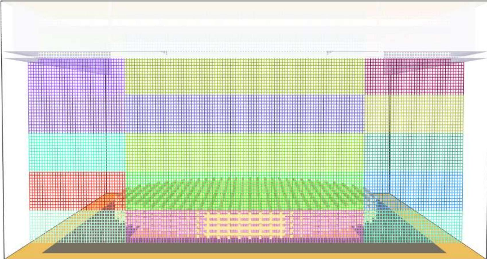
Multi-mesh in elevation view, mesh number 30 in total, cell size **0.03m×0.03m×0.035m** (to fit per cell - per cross section) for wood sticks, total number of cells 2,201,472 (HPC on ARCHER via UKCTRF)
