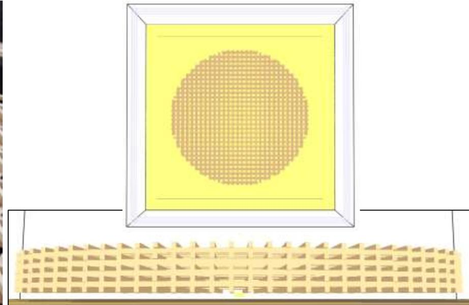
In the FDS model, we have no offset, hence less porosity (i.e. lower layers support reduced fire spread).
