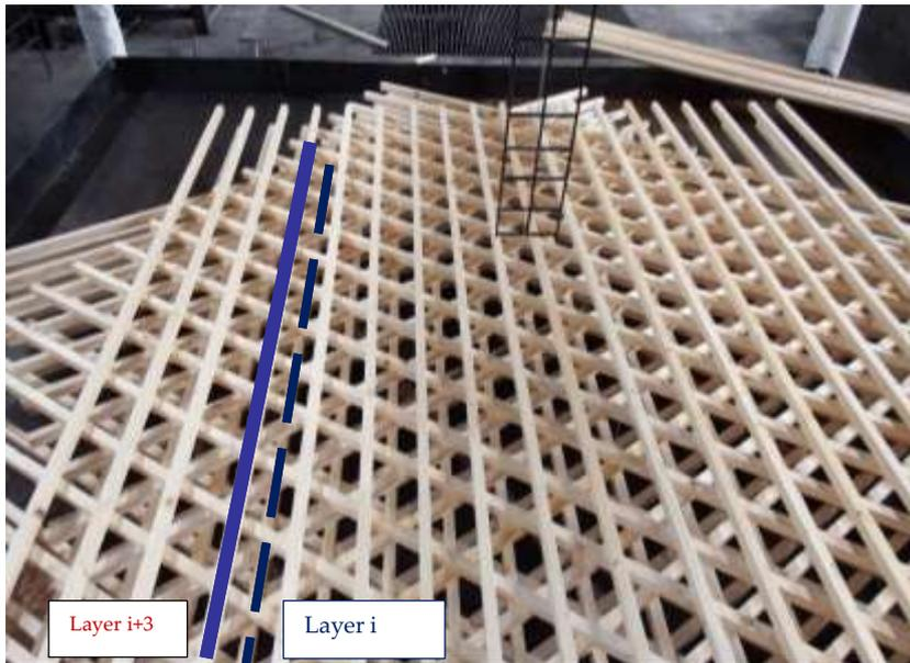
Shifted fuel load arrangement for test M7; Test M7 is made of 9 layers of sticks with an axis distance of 120 mm, layers  $i$  and  $i+3$  were shifted laterally by 60 mm.
