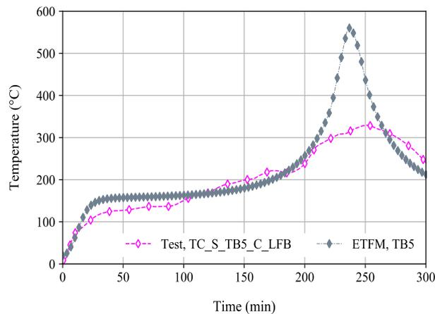
(f) TB6, bottom flange beam temperature
