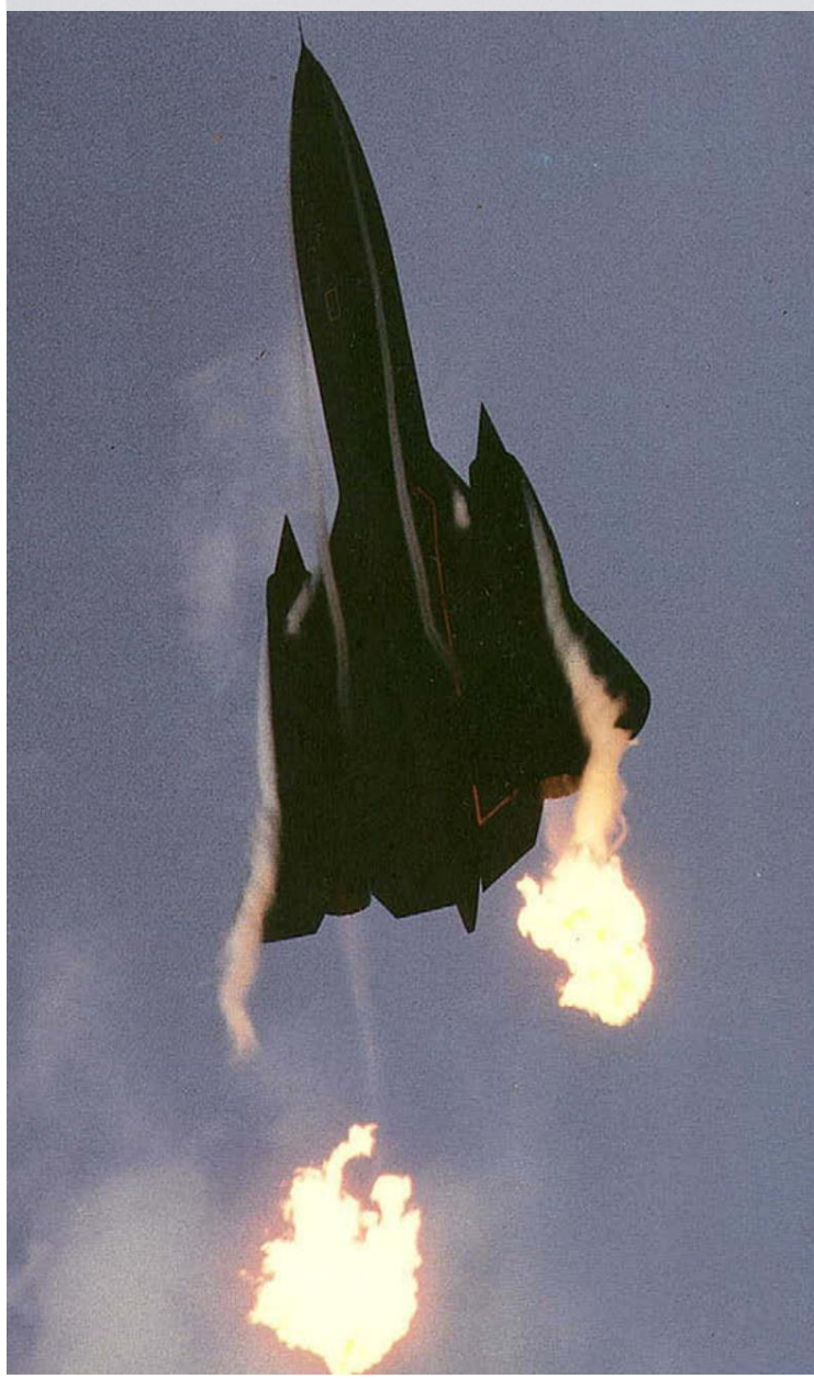
SR71 – afterburner blowout
