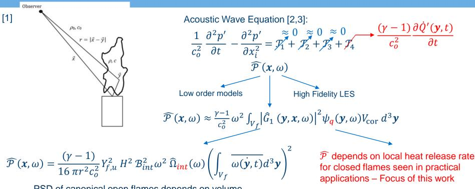
PSD of canonical open flames depends on volume integrated heat release rate (studied previously[4,5])
