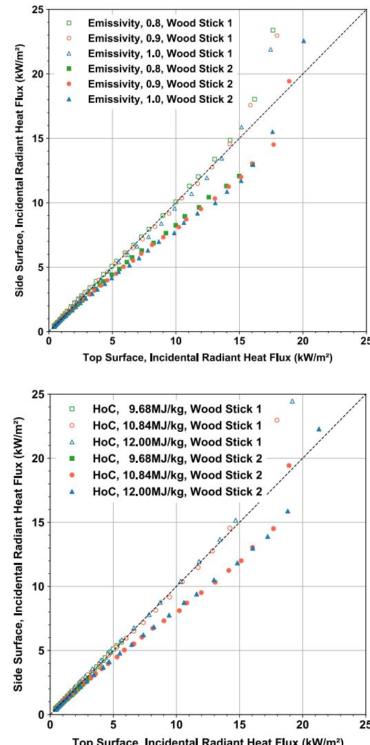
**Figure 26. Parameter sensitivity on heat flux comparison between top surface and side surface of wood sticks 1 and 2.**
