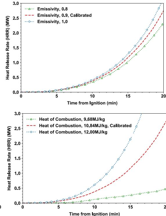
Figure 22. Parameter sensitivity on HRR: a) Ignition temperature of wood, b) Thermal inertia, c) Emissivity of wood, d) Soot concentration (prescribed), e) HRRPUA, f) Heat of Combustion
