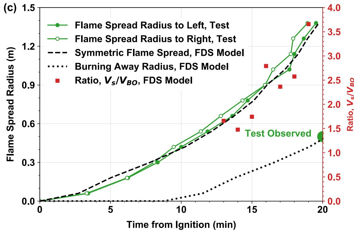
Figure 14. (c)  $V_s/V_b$ : velocity of flame spread front to velocity of flame burnout front.
