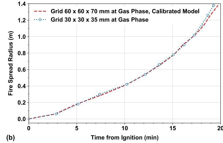
Figure 12. Cell size sensitivity at gas phase on (a) HRR, and (b) Fire spread radius.
