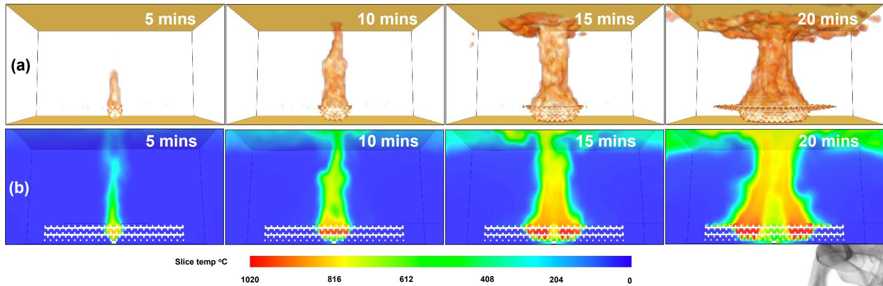
Figure 11. (a) Flame development within wood cribs (wood sticks “obstruction” removed in Smokeview for clearer flame demonstration), and (b) Temperature development at the compartment central ‘slice’.
