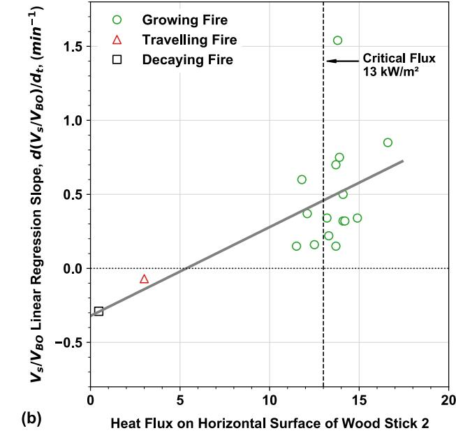
Figure 33. Relationship between fire modes development and heat flux on horizontal surface of (a) wood stick 1, and (b) wood stick 2, 1 min before ignition (summary all 19 cases).
