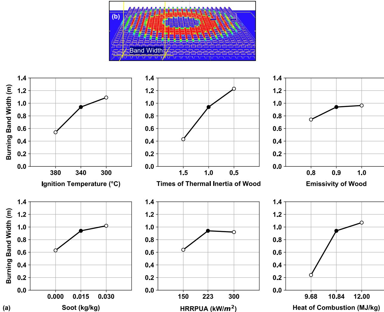
Figure 23. Maximum burning band width with 20 mins simulation (solid black dot: calibrated model).
