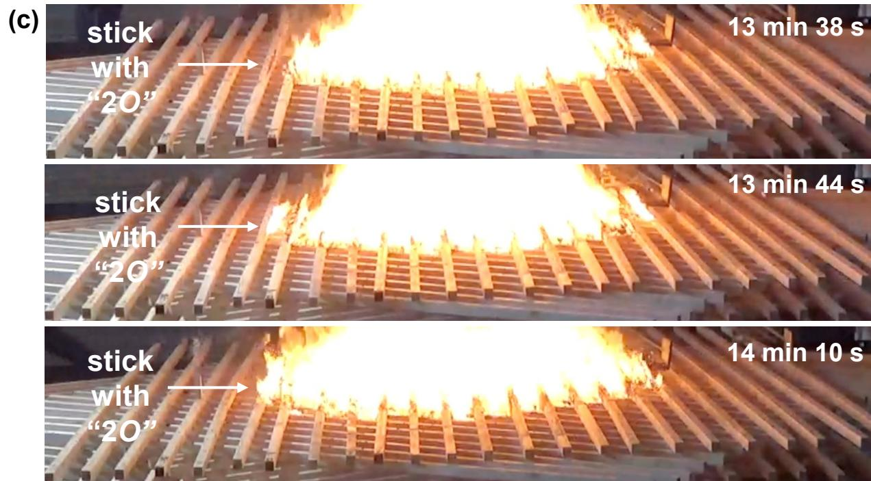
Figure 16. (c) Flame spread development on stick with thermocouple “2O”.
