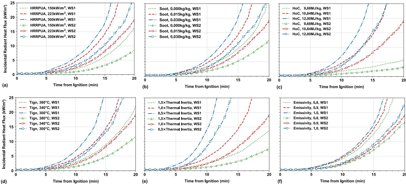
**Figure 25. Parameter sensitivity on incidental radiant heat flux at horizontal surface of wood stick 1 (WS1), and wood stick 2 (WS2).**
