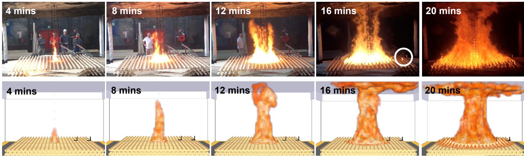
Figure 7. FDS simulated fire spread comparison with the test, at 4 mins, 8 mins, 12 mins, 16 mins, and 20 mins.
