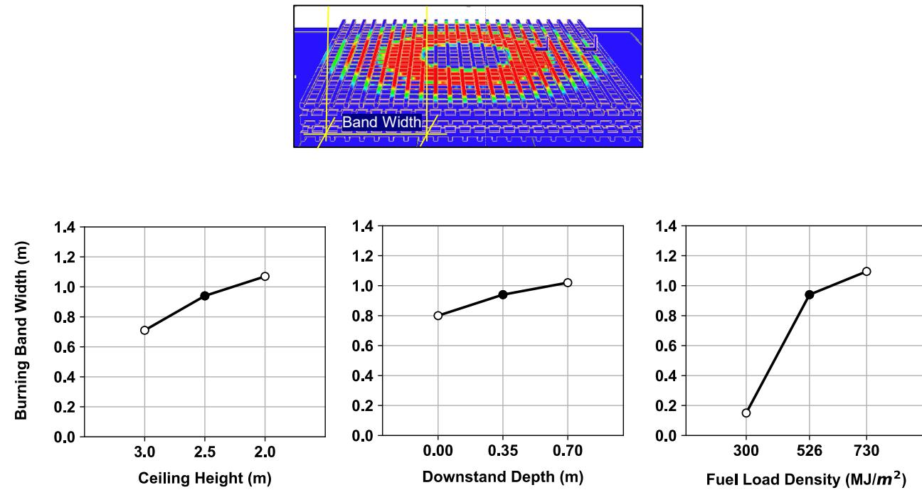
**Figure 29. Structural design parameter sensitivity on maximum burning band width with 20 mins simulation (solid black dot: calibrated model).**
