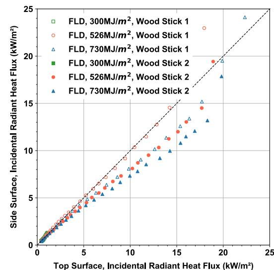
Figure 32. Structural design parameter sensitivity on heat flux comparison between top surface and side surface of wood sticks 1 and 2.
