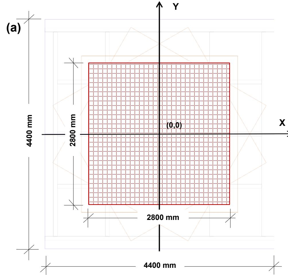
Figure 6. (a) Representation of the wood sticks in the model coordinate in plan view, simplified to a 2.8 m x 2.8 m square wood crib with sticks placed orthogonally.
