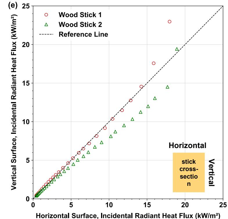
Figure 21. (a-d) Development of incidental radiant heat flux on top layer wood sticks, 13 kW/m<sup>2</sup> represented in black is critical heat flux for *Picea abies* wood ignition measured in Edinburgh fire lab using cone calorimeter, (e) Comparison of the heat fluxes on wood sticks 1 and 2 on horizontal surface vs. vertical surface.
