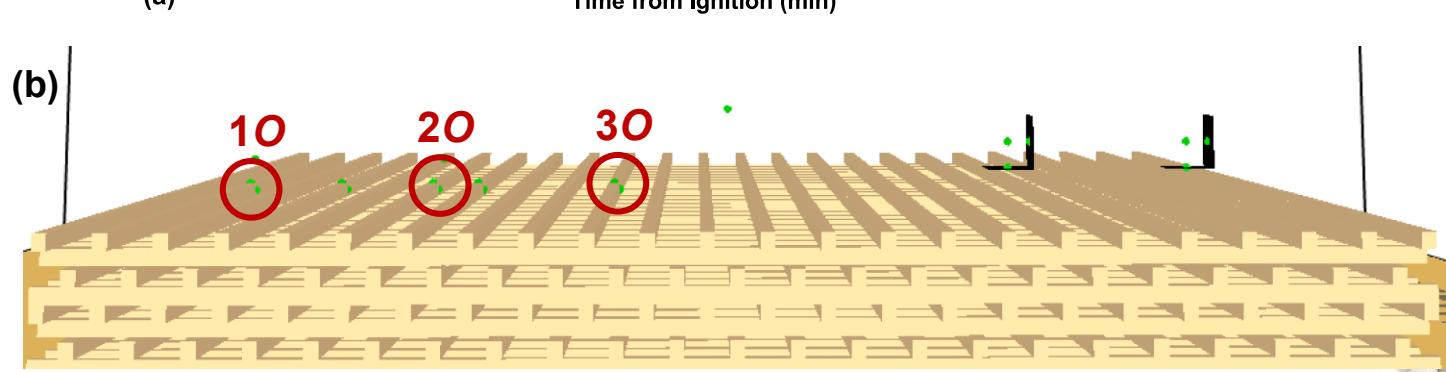
Figure 15. (a) Comparison of thermocouple temperatures on wood sticks top layer between model and test, and (b) Thermocouple instrumentation locations in model.
