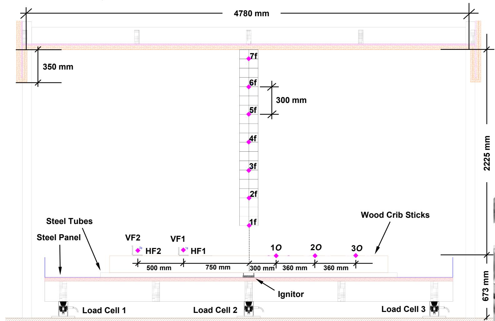
Figure 2. Overview of test setup in elevation: compartment structure, plate thermometer and thermocouple instrumentations (marked with pink square dot), and location of sticks.
