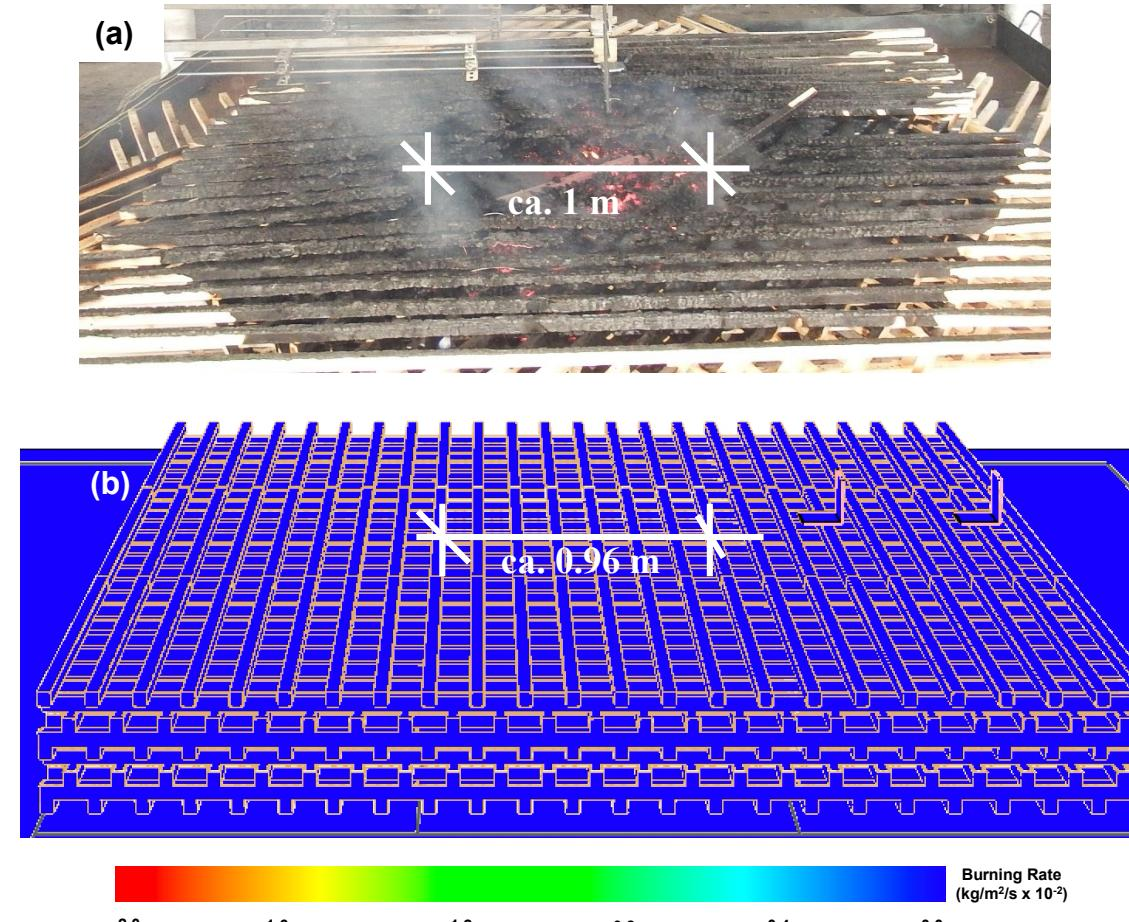
Figure 13. Burning away comparison between (a) the LB7 post-test photo, and (b) the model on burning rate at 20 mins.
