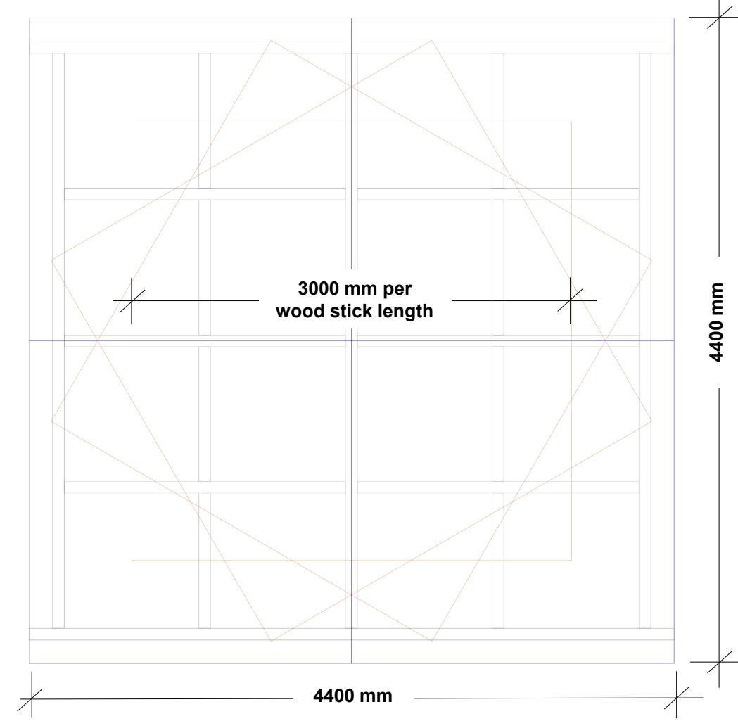
Figure 4. Test setup in plan view: wood stick orientation shifted  $60^\circ$  per layer.
