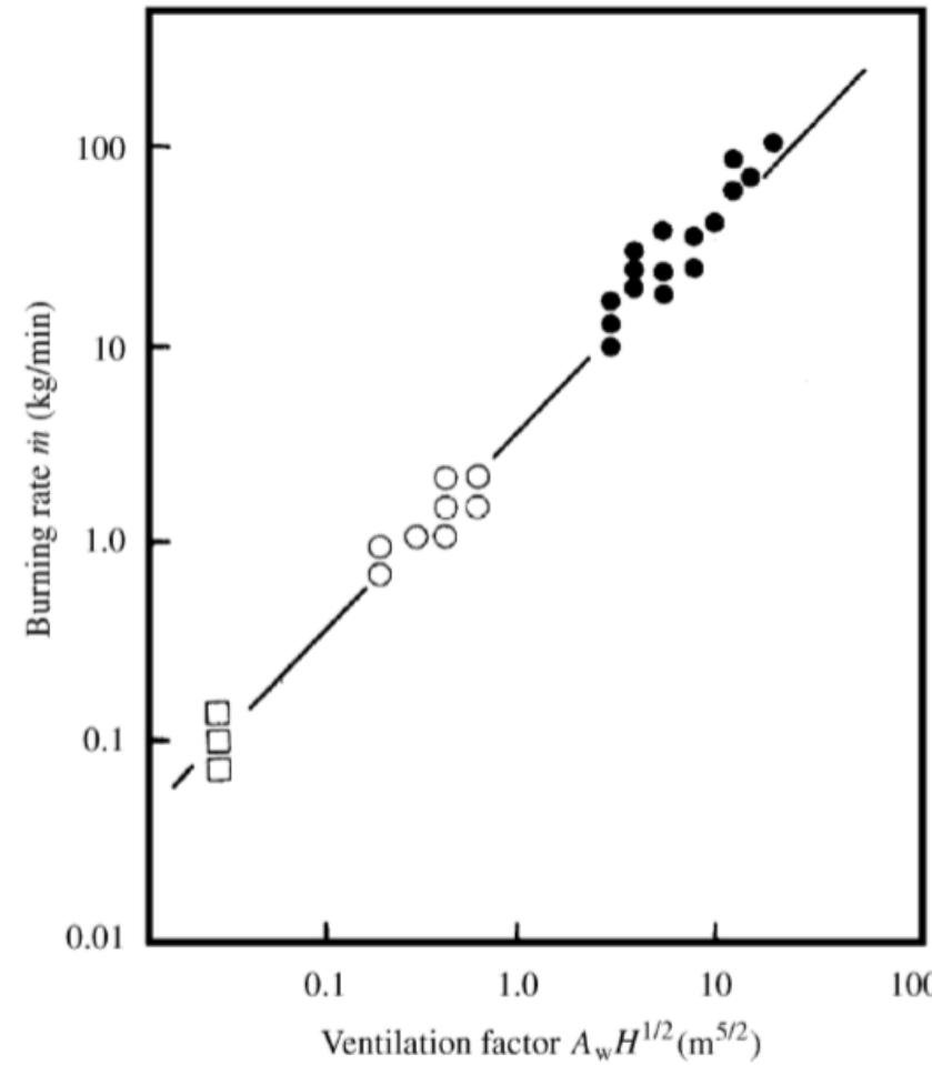
**Figure 10.1** Mass burning rate of wood cribs in enclosures as a function of the ventilation factor,  $A_w H^{1/2}$  for ventilation-controlled fires (Equation (10.1)): ●, full-scale enclosures; ○, intermediate-scale models; □, small-scale models (Kawagoe and Sekine, 1963). Reproduced by permission of Elsevier Applied Science Publishers Ltd
