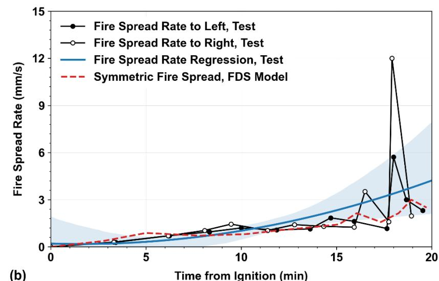
Figure 8. Comparison between the test and the model, (a) Fire spread radius from wood crib centre to edge, and (b) Fire spread rate from wood crib centre to edge.
