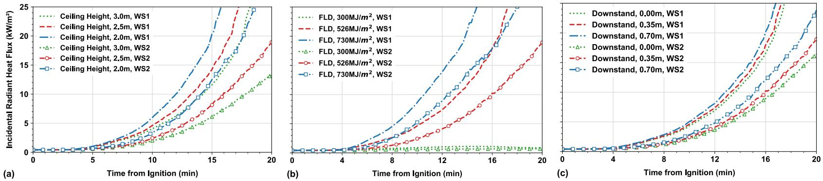
**Figure 31. Design parameter sensitivity on incidental radiant heat flux at horizontal surface of wood stick 1 (WS1), and wood stick 2 (WS2).**
