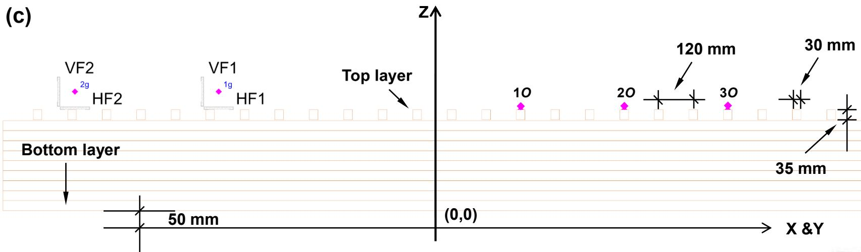
Figure 6. (c) Representation of the wood sticks in the model coordinate in elevation view, stick size 35 mm x 30 mm with stick pitch 120 mm, 24 sticks per layer, 9 layers in total, and 50 mm offset between the steel panel and the bottom wood stick layer for the ignition burner and steel tubes.
