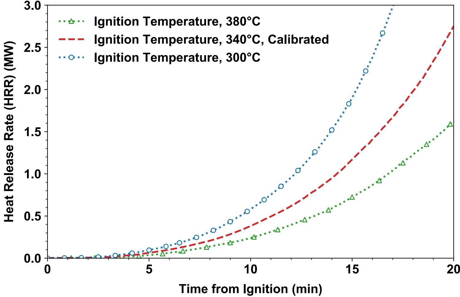
Figure 22. Parameter sensitivity on HRR: a) Ignition temperature of wood
