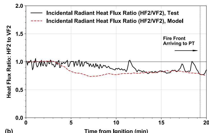
Figure 20. Comparison between test and model on incidental radiant heat flux ratio of (a) HF1 to VF1, and (b) HF2 to VF2.
