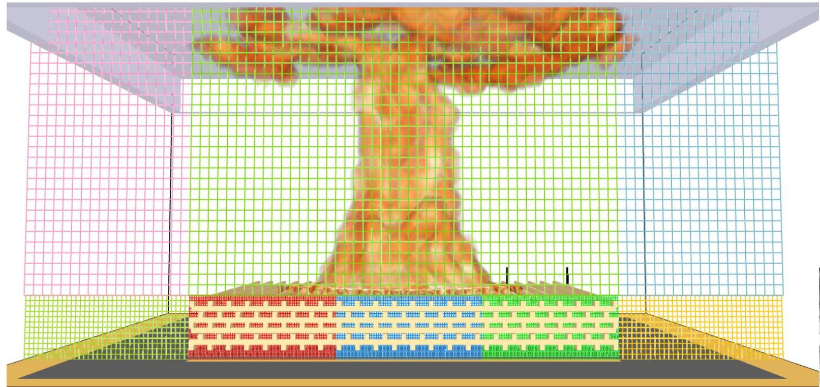
Figure 5. Grid cell resolution of the model:  $1.5\text{ cm} \times 1.5\text{ cm} \times 1.75\text{ cm}$  per cell for wood sticks in porous crib structure,  $6\text{ cm} \times 6\text{ cm} \times 7\text{ cm}$  and  $3\text{ cm} \times 3\text{ cm} \times 3.5\text{ cm}$  cell size in gas phase, total number of cells  $\sim 1.3$  million.
