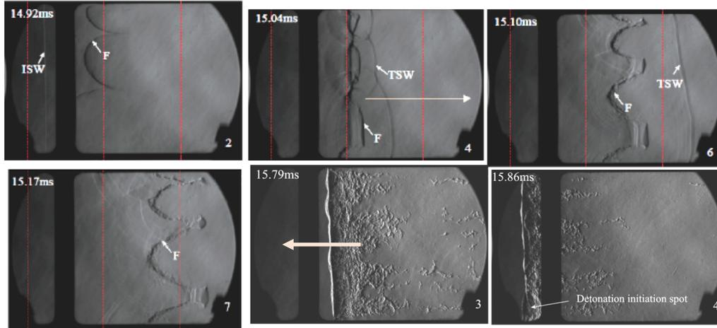
FSI,  $P=17\text{kPa}$ ,  $Ms = 1.9$ ,  $\phi = 1$ , Rectangular Tube : 20cm high
