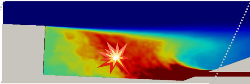
Averaged Fuel air equivalence ratio snapshots at the center plane of the injector and the center plane between two injectors without combustion
