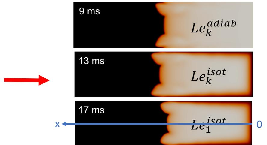
Flame front position on symmetry axis
