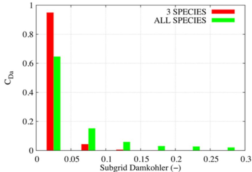
Cell ratio in each interval of subgrid Damköhler number.
