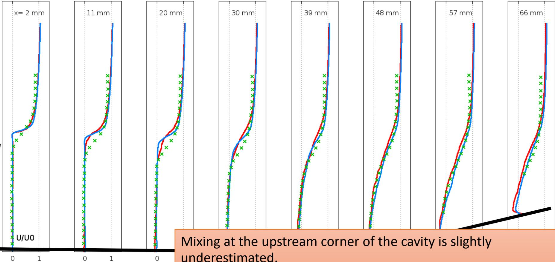
Mixing at the upstream corner of the cavity is slightly underestimated.
