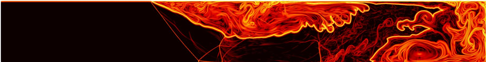
Ms=1.9, ISOTHERMAL WALLS, Complex Transport / gradient of total energy
