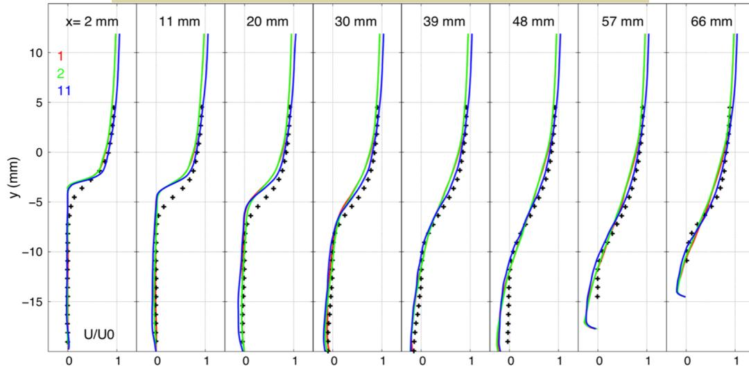
Very few impact on the averaged cavity wall pressure and streamwise velocity (taken between 6<sup>th</sup> and 7<sup>th</sup> injector for the case 11 inj.)
