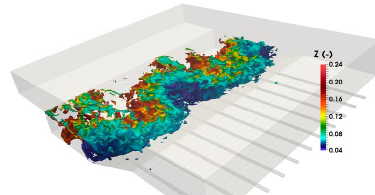
Instantaneous isosurface of temperature at 2000 K colored by the values of mixture fraction
